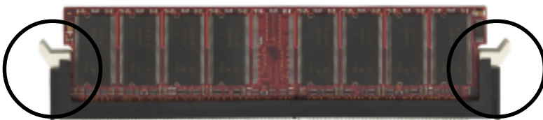
Figure 9 - DIMM module clip after installation
