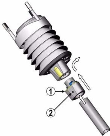
**Figure 9**      **Mounting WXT510 to Pole Mast Using Optional Mounting Kit**
