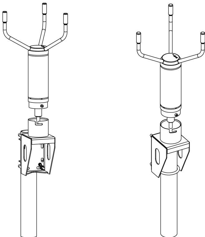
When mounting WMT700 on a cross arm, the wind sensor can be placed with the array facing up or down. The following figure shows WMT700 installed with the array facing up. If the wind sensor is installed with the array facing down, refer to section Configuration Parameters in the User's Guide.
