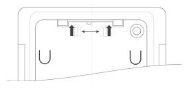
**Step 5** Before re-attaching the logger to the vNet device, inspect the vNet connector for any misaligned or bent pins. If you find misaligned or bent pins, contact support as per the information below.
