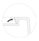
Step 4 Press the spacer firmly against the wall so that it adheres in place.
