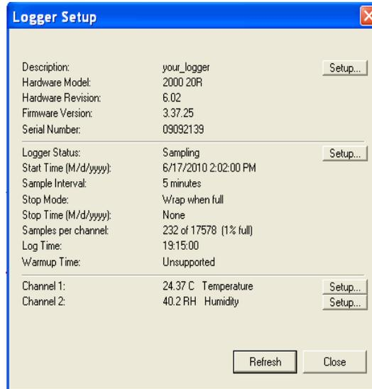
The information shown in the Logger Setup window relates to the data logger connected to the COM port you have specified. Some fields shown will vary depending on the model of data logger in use.
