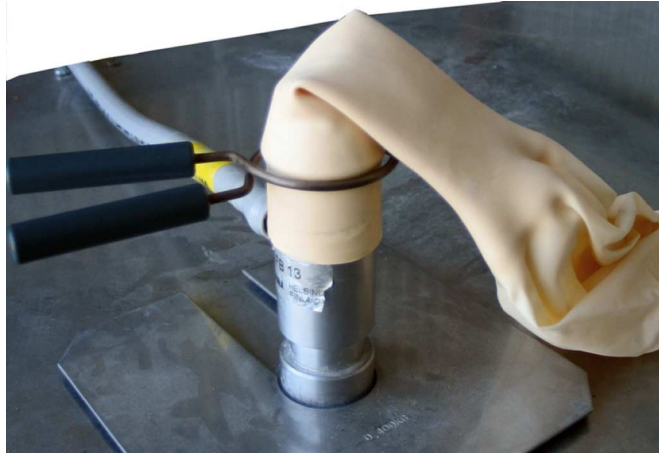
Figure 3 Attaching the Balloon to the Gas Nozzle
