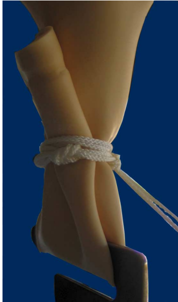
Figure 8 Folding the Neck of the Balloon
