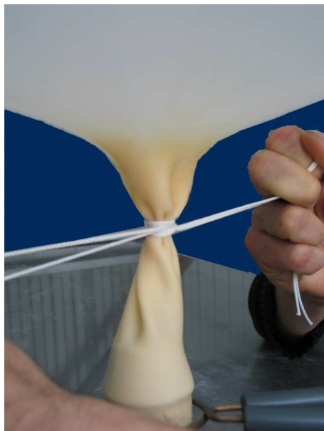
Figure 6 Securing the Neck of the Balloon
