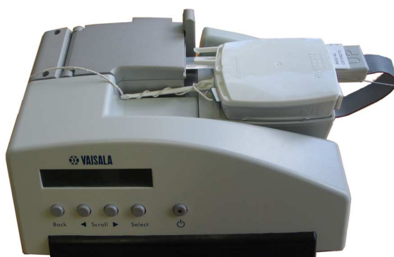
Figure 14 Radiosonde in the GC25 with the Communication Cable Connected
