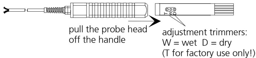
**FIGURE 6-2** Adjustment trimmers and probe head connection/disconnection
