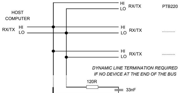
At the ends of the serial bus there must be a PTU200 series transmitter, a dynamic line adapter (120 ohm resistor in series with a 33 nF capacitor) or a line master. If a branch line is made with a junction box, the branch should be shorter than 3 meters.
