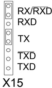
**FIGURE 4-2** RS 232C/TTL level and phase selections
