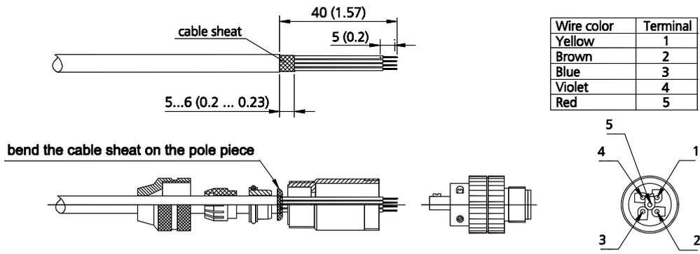
**FIGURE 3-4** Connecting the cable. Dimensions in mm (inches).
