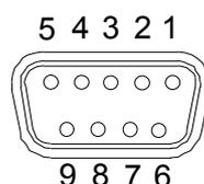
FIGURE 3-1 9-pin female sub D-connector
