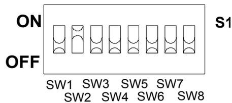
**FIGURE 4-4** External power control ON
