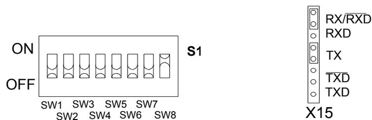
**FIGURE 7-1** Factory settings for the dip switch S1 and Basic RS 232C settings
