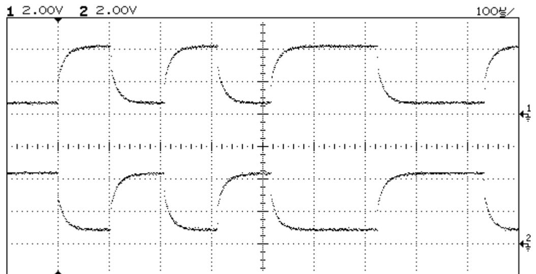
The next picture (below) shows typical RS485/422 differential output signals RS485/422 LO (upper signal) and RS485/422 HI (lower signal) at baud rate 9600. The vertical scale is 2V/div for both signals. The ground level for each signal is shown with a small arrow at the right. At the left the signals are at rest.
