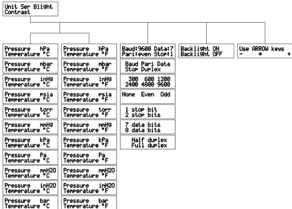
FIGURE 4-1 Available functions and selections of the local display
