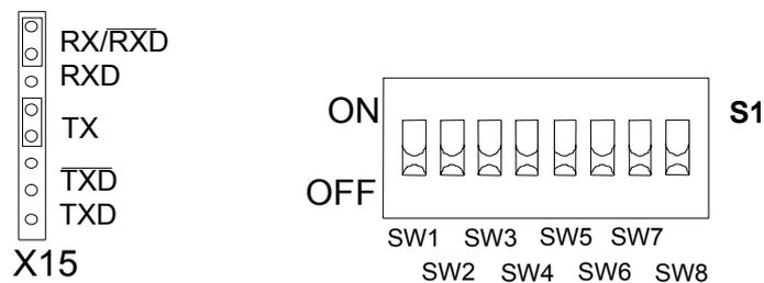
**FIGURE 3-2** Basic RS 232C jumper and dip switch S1 settings
