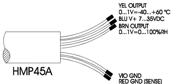
**FIGURE 3-3** Wire colours of HMP45A-P.
