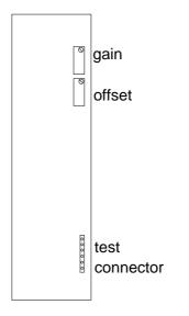
Figure 2.4 Calibration connector and potentiometers in the HMW 20/30UB/YB transmitters
