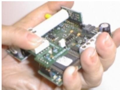
**Figure 2 Installing the GMR20 module**
