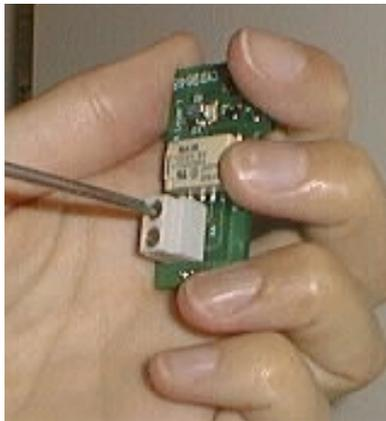
**Figure 1 Connecting the wires to the GMR20 module**
