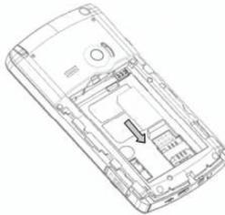
4. Replace the battery and gently push down to snap it into place.
