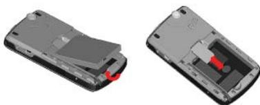
4. Replace the battery and gently push down to snap it into place.
