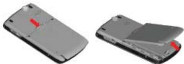
3. Proceed to remove the battery first. Then, insert the SIM card into the SIM card slot with its gold contacts facing down (the cut-off corner of the SIM card should match the cut-off corner in the slot).
