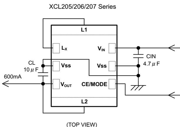
\* "L1 and L<sub>x</sub>", and "L2 and V<sub>OUT</sub>" is connected by wiring.
