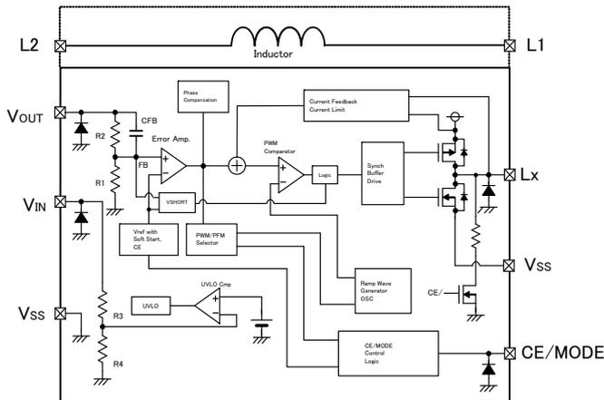
NOTE: The XCL205 offers a fixed PWM control, a signal from CE/MODE Control Logic to PWM/PFM Selector is fixed to "L" level inside. The XCL206 control scheme is PWM/PFM automatic switching, a signal from CE/MODE Control Logic to PWM/PFM Selector is fixed to "H" level inside. The diodes placed inside are ESD protection diodes and parasitic diodes.
