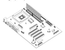
Note: You must install at least one memory module in order to have the mainboard work properly, either SDRAM or DDR SDRAM, but you can't use them simultaneously.
