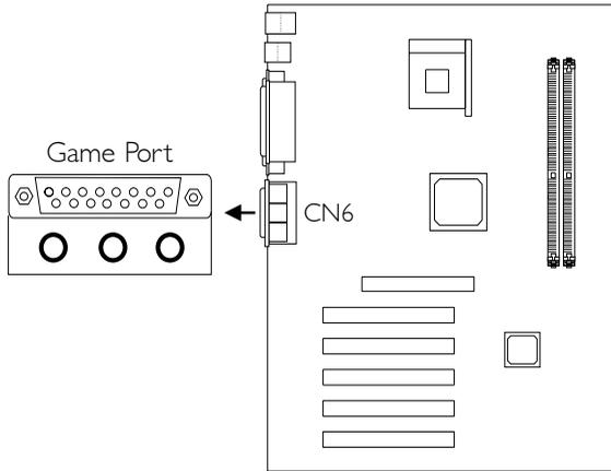
The Game/MIDI port is identical to that of a standard PC game adapter or game I/O port. Connect an analog joystick to the 15-pin D-sub connector (CN6 - Gold) located at the ATX double deck ports of the system board. This port works well with any application that is compatible with the standard PC joystick. You can configure the game port in the Integrated Peripherals submenu of the BIOS.
