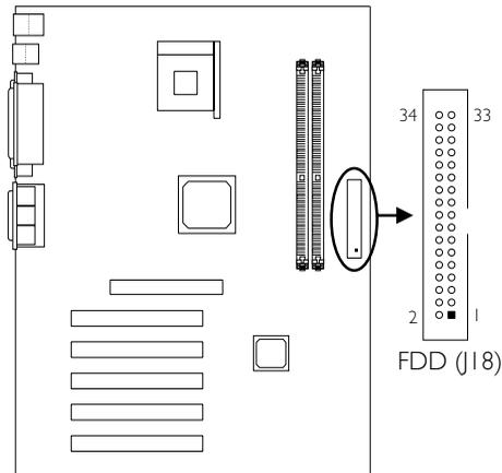
The system board is equipped with a shrouded floppy disk drive connector that supports two standard floppy disk drives. To prevent improper floppy cable installation, the shrouded floppy disk header has a keying mechanism. The 34-pin connector on the floppy cable can be placed into the header only if pin 1 of the connector is aligned with pin 1 of the header. You can enable or disable this function in the Integrated Peripherals submenu of the BIOS.
