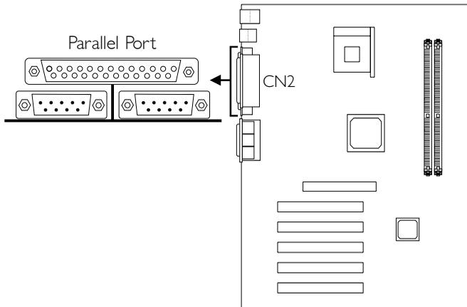
The system board has a standard parallel port (CN2 - Burgundy) located at the ATX double deck ports of the board for interfacing your PC to a parallel printer. It supports SPP, ECP, EPP and PntMode modes. You can select the port's mode in the Integrated Peripherals submenu of the BIOS.
