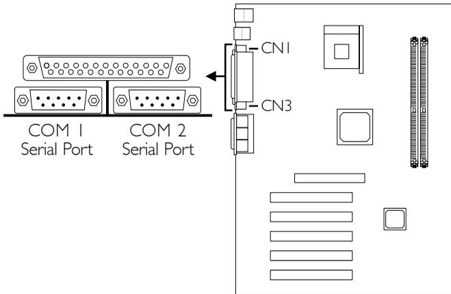
The system board is equipped with onboard serial ports (COM 1: CN1 and COM 2: CN3) - both in Teal/Turquoise color located at the ATX double deck ports of the board.
