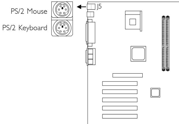
The system board is equipped with an onboard PS/2 mouse (Green) and PS/2 keyboard (Purple) ports - both at location J5 of the ATX double deck ports of the system board. The PS/2 mouse port uses IRQ12. If a mouse is not connected to this port, the system will reserve IRQ12 for other expansion cards.
