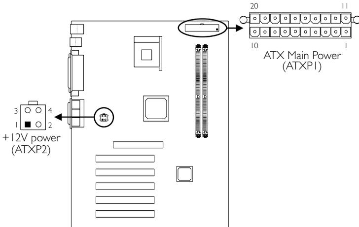
We recommend that you use a power supply that complies with the ATX12V Power Supply Design Guide Version 1.1. An ATX12V power supply has a standard 20-pin ATX main power connector and a 4-pin +12V power connector that must be inserted onto ATXP1 and ATXP2 connectors respectively.
