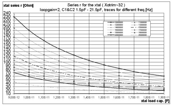
Figure 14. ESR vs. Load Capacitance for the Crystal
