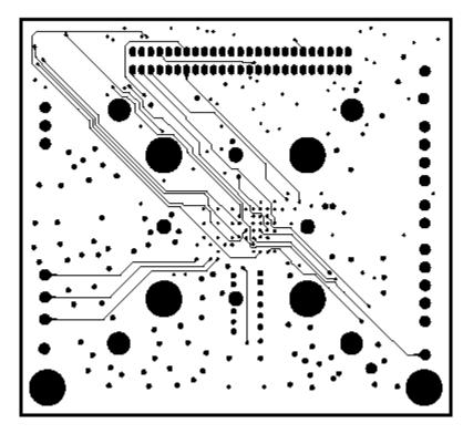
Figure 25. Signal Plane (Layer 3)
