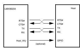
Figure 17. UART Null Modem Connections
