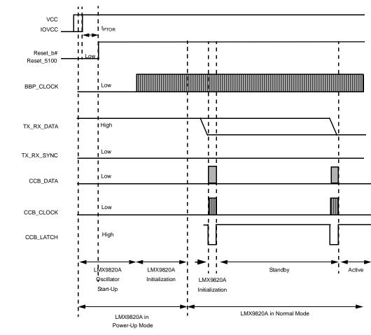
Figure 15. LMX9820A System Power-Up Sequence Timing
