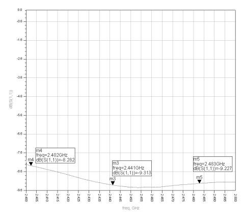
Figure 9. Transceiver Return Loss
