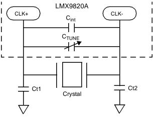
Figure 10. LMX9820A Crystal Recommended Circuit
