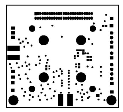
Figure 26. Component Layout Bottom (Layer 4)
