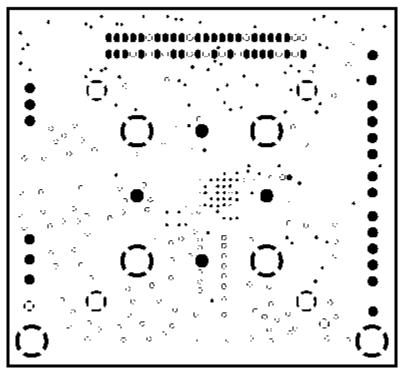
Figure 24. Solid Ground Plane (Layer 2)
