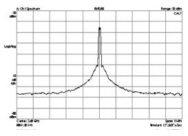
Figure 6. Synthesizer Phase Noise
