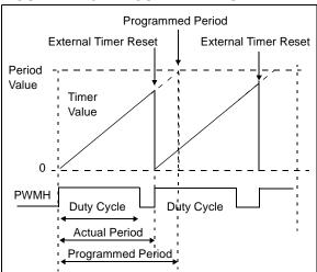
Typically, in the converter application, an energy storage inductor is charged with current while the PWM signal is asserted, and the inductor current is discharged by the load when the PWM signal is deasserted. In this application of current reset PWM, an external current measurement circuit determines when the inductor is discharged, and then generates a signal that the PWM module uses to reset the time base counter. In Current Reset mode, complementary outputs are available.
