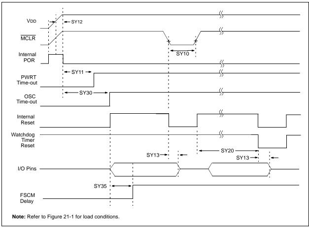
TABLE 21-18: RESET, WATCHDOG TIMER, OSCILLATOR START-UP TIMER, POWER-UP TIMER AND TIMING REQUIREMENTS
