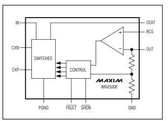
low-impedance trace, and connect the ground for  $C_{\rm IN},$   $C_{\rm EXT},$  and  $C_{\rm OUT}$  directly to PGND in a star configuration. Connect R\_CS to C\_{\rm EXT} through a short and low impedance trace.
