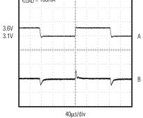
A: INPUT VOLTAGE: 500mV/div B: OUTPUT VOLTAGE: AC-COUPLED, 100mV/div
