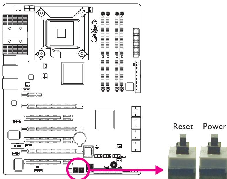
The presence of the power switch and reset switch on the system board are user-friendly especially to DIY users. They provide convenience in powering on and/or resetting the system while fine tuning the system board before it is installed into the system chassis.
