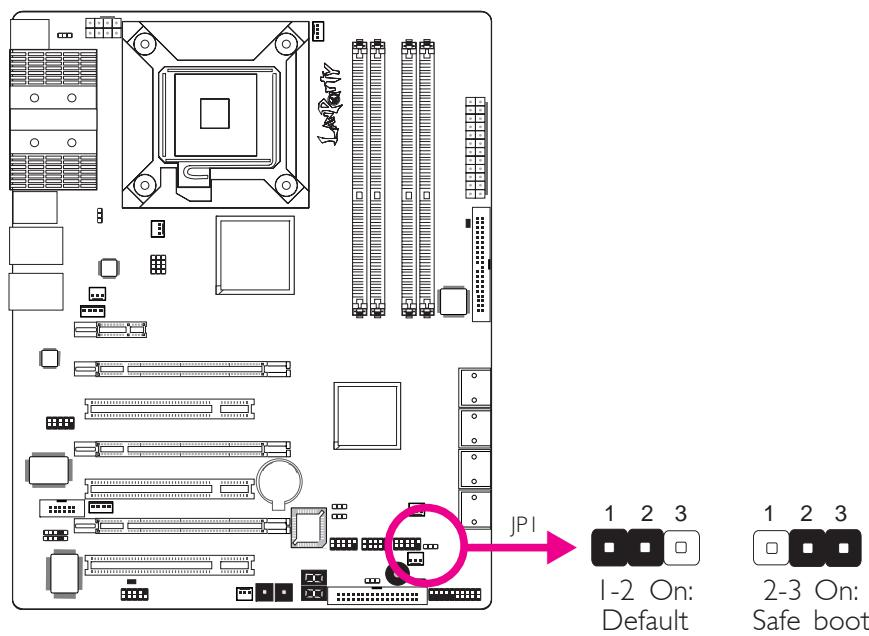
This jumper is used to safely reboot the system whenever the system hangs and you are unable to restart the system.
