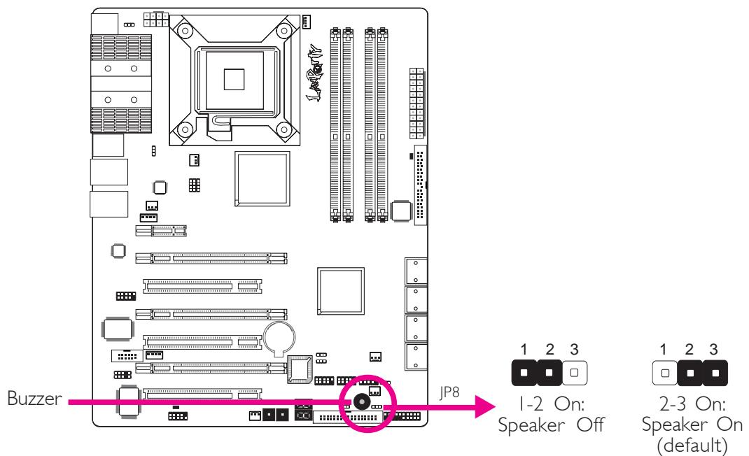
The system board is equipped with a buzzer which serves as the PC's speaker. By default the buzzer is “on” allowing you to hear the system's beep messages and warnings. If you intend to use an external speaker, turn this function off by setting JP8 pins 1 and 2 to On.
