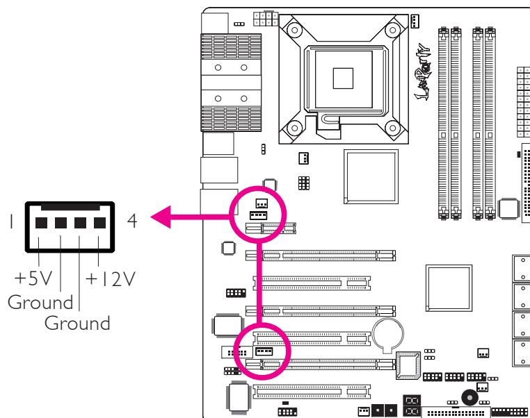
The system board requires a minimum of 300 Watt power supply to operate. Your system configuration (CPU power, amount of memory, add-in cards, peripherals, etc.) may exceed the minimum power requirement. To ensure that adequate power is provided, **we strongly recommend that you use a minimum of 400 Watt (or greater) power supply.**
