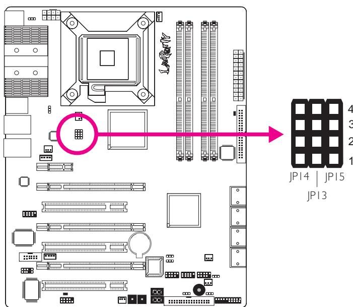
By default, JP13 to JP15 are set to pins 1 and 2 On. This setting will allow the system to automatically run according to the CPU's FSB. If you want to change the setting, please refer to the table below.
