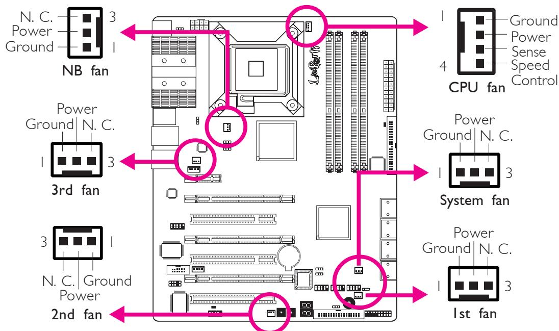
These fan connectors are used to connect cooling fans. Cooling fans will provide adequate airflow throughout the chassis to prevent overheating the CPU and system board components.
