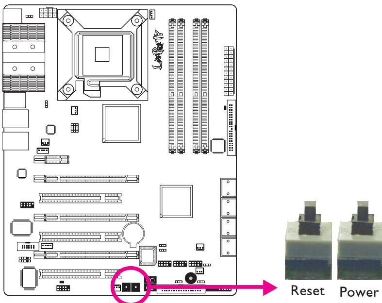
If the system board is already enclosed in a chassis, apply the same method using the Reset button and Power button located at the front panel of the chassis.
