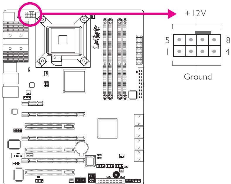
The power connectors from the power supply unit are designed to fit the 24-pin and 8-pin connectors in only one orientation. Make sure to find the proper orientation before plugging the connectors.
