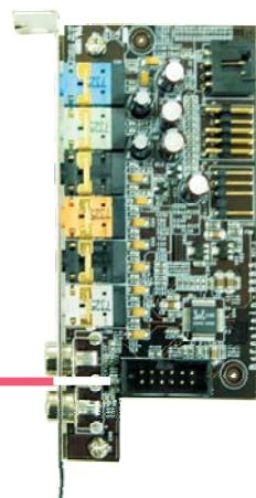
3. The length of the audio cable provides the option and flexibility of installing the module on any available expansion bracket slot at the rear of the system chassis. Remove the screw of the bracket where you want the audio module installed then remove the bracket. Place the Bernstein audio module on the expansion bracket slot then secure the module by replacing the bracket screw you removed earlier.
