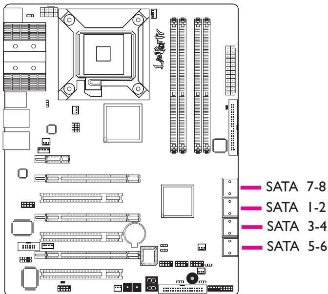
The Serial ATA (SATA) connectors are used to connect Serial ATA drives. Connect one end of the Serial ATA cable to a Serial ATA connector and the other end to your Serial ATA device.
