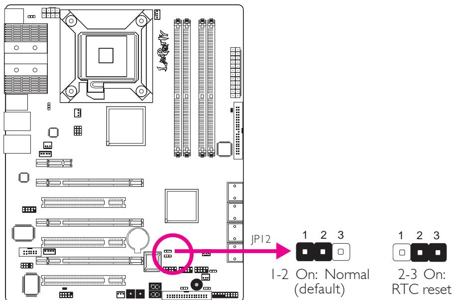
When the RTC battery is removed, this jumper resets the manageability register bits in the RTC.
