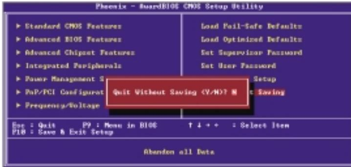
Type "Y" and press <Enter>. The system will reboot and you will once again see the initial diagnostics on the screen. If you wish to make any changes to the setup, press <Ctrl> <Alt> <Esc> simultaneously or <Del> after memory testing is done.
