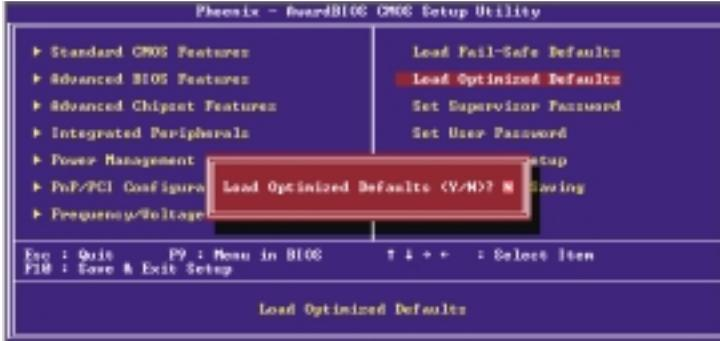
Type <Y> and press <Enter> to load the Setup default values.
