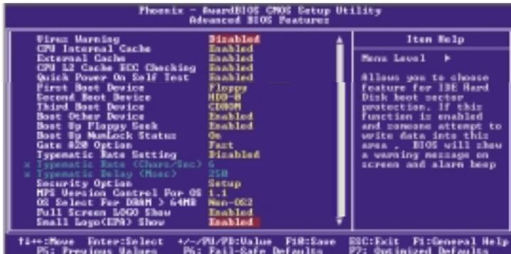
The screen above list all the fields available in the Advanced BIOS Features submenu, for ease of reference in this manual. In the actual CMOS setup, you have to use the scroll bar to view the fields. The settings on the screen are for reference only. Your version may not be identical to this one.
