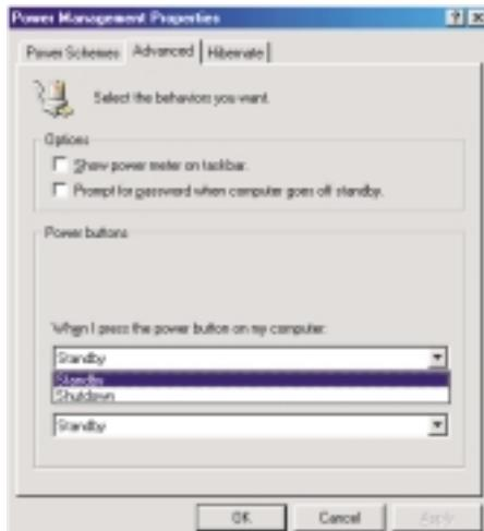
12. After completing the steps above and you want to power-off the computer; you do not need to go through the process of closing files, applications and operating system. You can power-off the computer at once by pressing the power button or selecting "Standby" when you shut down Windows® 98.
