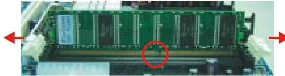
3. Lower the RAM module into the DIMM Slot and press firmly using both thumbs until the module snaps into place.
