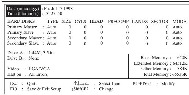
1. Select "Standard CMOS Setup" in the main program screen and press <Enter>.
