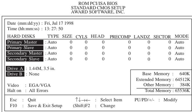
1. Select “Standard CMOS Setup” in the main program screen and press <Enter>.
