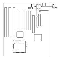
connectors J4 and J5. Mount the cardedge bracket to the system chassis.
