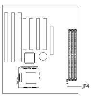
compatibility problems with PC-100 SDRAM DIMMs or you are using EDO / PC-66 SDRAM DIMMs, set the SDRAM clock according to the AGP clock (1-2 On).
