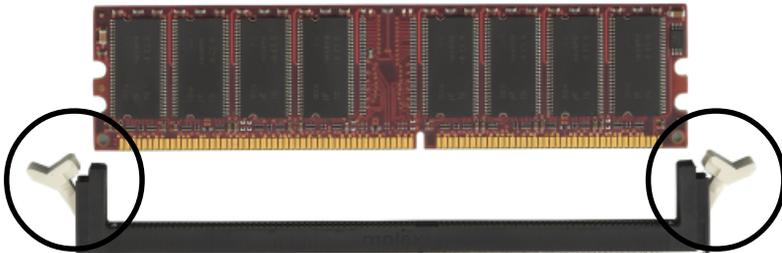
*Figure 9 - DIMM module clips before installation*
