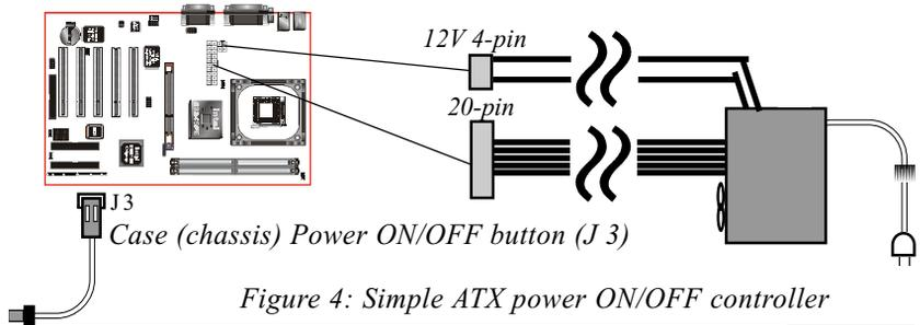
Figure 4: Simple ATX power ON/OFF controller
