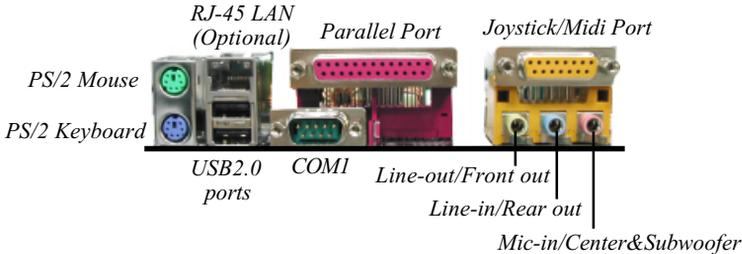
Figure 11 - I/O Ports
