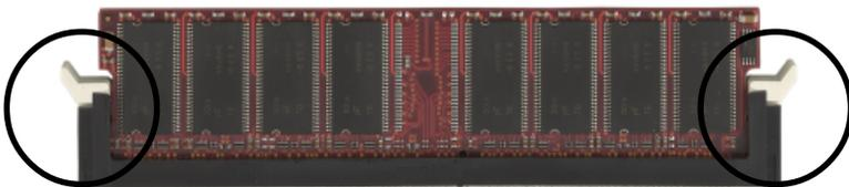
*Figure 10 - DIMM module clip after installation*
