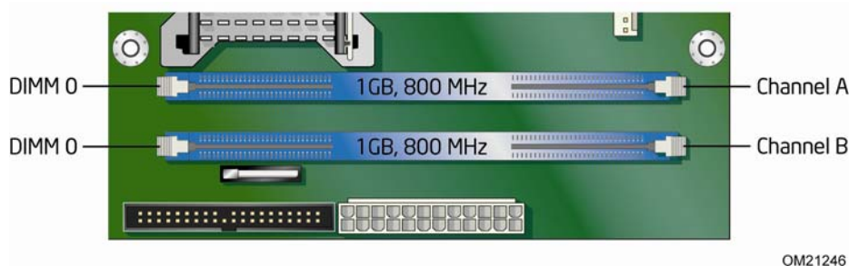
Figure 13. Dual Channel Memory Configuration Example
