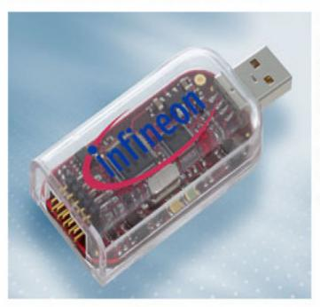
The XC164CM U CAN start kit supports debug of the 16bit MCU via a USB-JTAG solution. The TwinCAN feature of the XC164CM includes 2 CAN transceivers allowing both CAN nodes to be accessed through a 10-pin header, which also allows access to analog and digital VO signals. The kit comes with a dedicated CAN application program already loaded into the embedded flash memory of the XC164CM MCU, supported with an Application GUI, allowing for easy demonstration of the CAN features.
