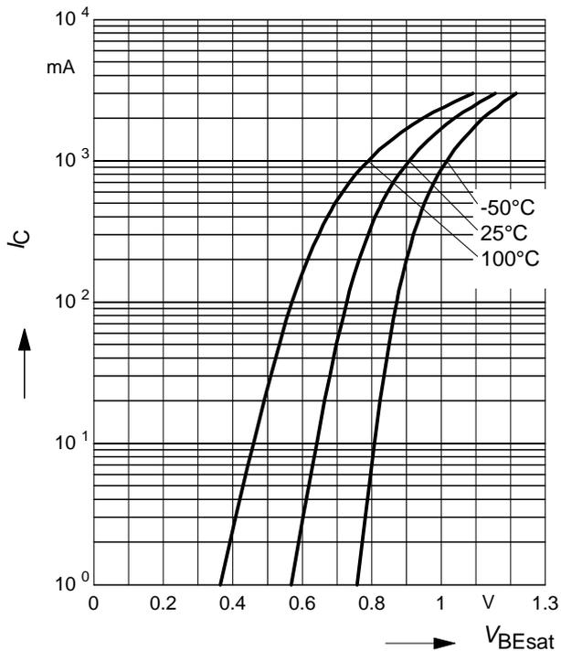
**Collector current  $I_C = f(V_{BE})$**
