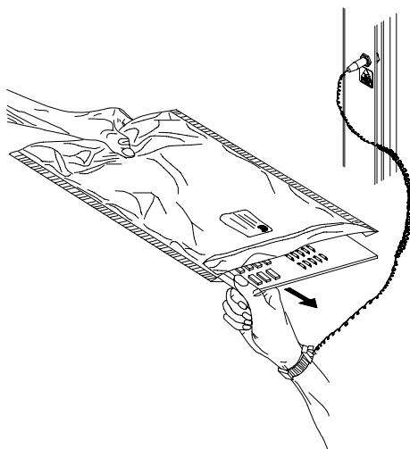
**Figure 3-1** Diagram of wearing electrostatic protection wrist strap
