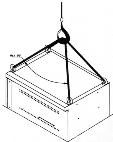
**Figure 3-2 Weight hoisting**
