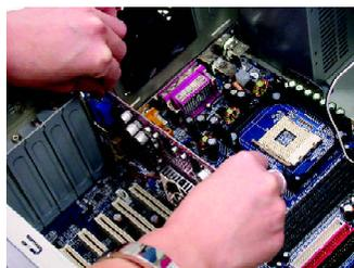
4. Locate the AGP slot. If necessary, remove the metal cover from this slot; then align your Graphics card with the AGP slot, and press it in firmly until the card is fully seated.
