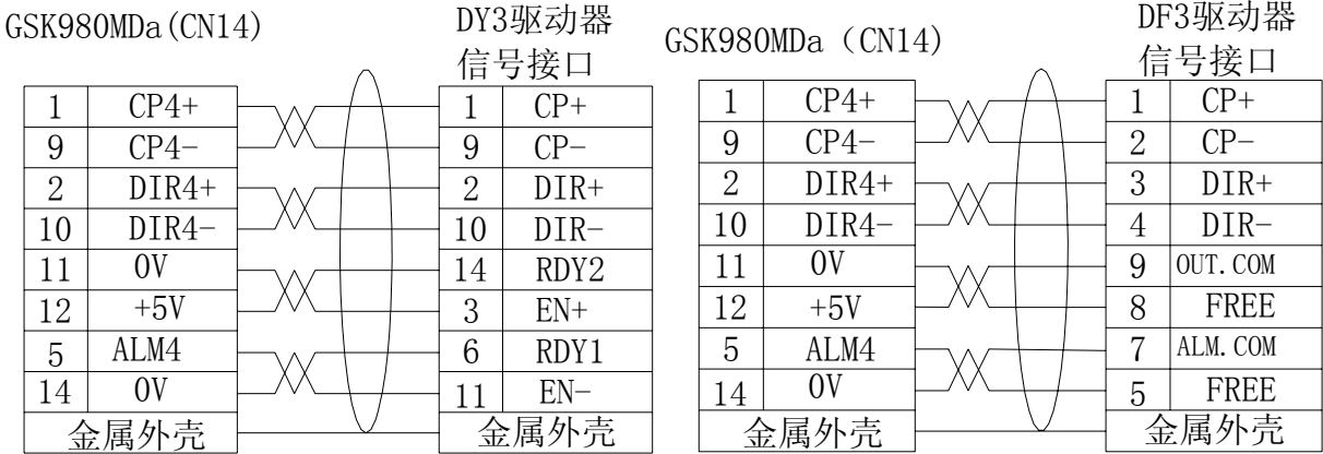
图 2-12 4th 轴接口与驱动单元的连接
