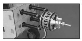
4. Select the mount base/spacer/bolt combination necessary to extend your motor the correct distance from the fireweall. Apply a few drops of threadlocker to the threads on the end of the mounting bolts. Then, mount your motor using #8 lock washers and #8 flat washers under the heads of the bolts
