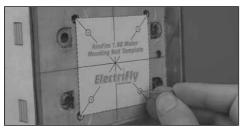
1. Use the RimFire<sup>™</sup> 1.60 motor mounting bolt template to mark the bolt hole locations on your firewall.
