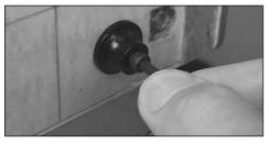
3. Use a 9/64" hex wrench to draw the blind nuts into the back of the firewall with one of the mount bases and an 8-32 bolt. Optional: Apply thin or medium CA around each blind nut to permanently hold it into the back of the firewall—use care **NOT** to get any CA into the threads.
