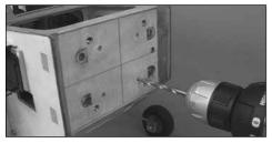
2. First, drill 1/16" [1.6mm] guide holes through the firewall at the marks you made with the template. Then, enlarge the guide holes with a 7/32" [5.5mm] drill to accommodate the blind nuts.
