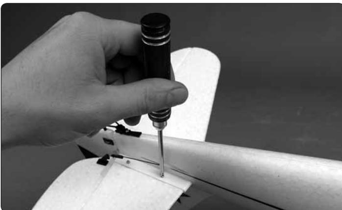
❑ 3. Slide the two horizontal stabilizer halves into the fuselage so that the carbon pins installed in one side fit into the mating holes in the other side and that the elevator joiner fits into
