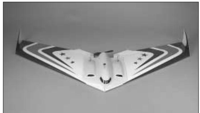
❑ 2. Glue the wing tips to the wing with 6-minute epoxy.
