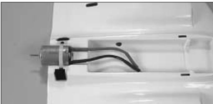
3. Secure the motor to the center section with the included nylon tie strap. Notice that the wires have already been soldered to the motor.
