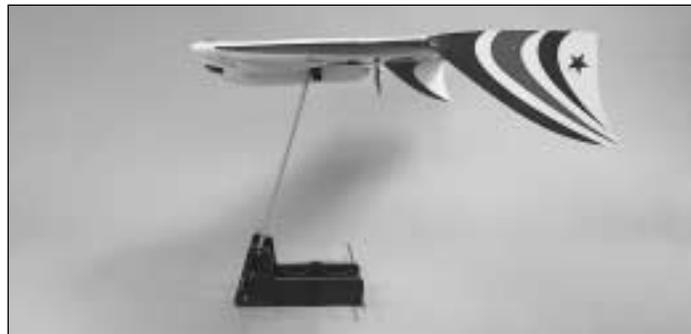
□ 2. Lift the model, upside down, at the balance point you marked on the top of the wing. In the photo, we are using a Great Planes CG Machine™. If the nose drops the model is nose-heavy and you must add weight to the tail. If the tail drops, the model is tail-heavy and you must add weight to the nose. In most cases you can relocate the receiver to achieve the correct balance without adding more weight.
