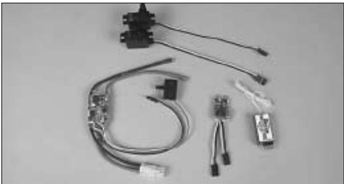
The Slinger requires a three-channel radio with two servos, a receiver, mixer and a speed control. A small receiver and mini servos are required, and smaller radio equipment designed for park flyer models can be used. The servos must have a minimum of 15 oz-in torque.
