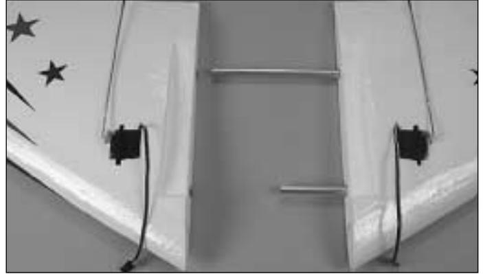
□ 1. Insert the aluminum joiner tubes into the left wing panel. The longer tube goes in the rear hole.
