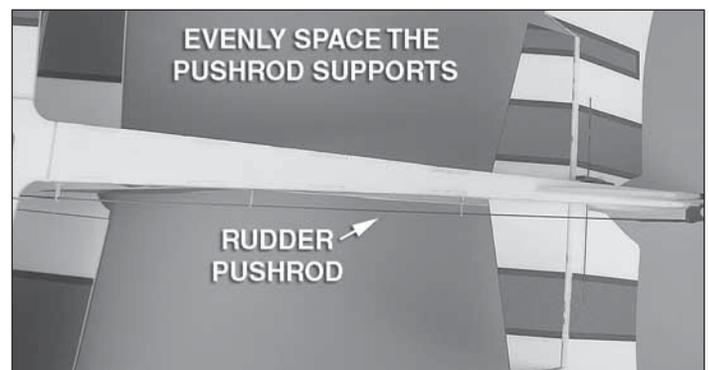
5. With the pushrod straight, cut 2mm wide slots in the fuselage for the pushrod supports using a hobby knife. Cut the first slot so that it is 5-1/2" [140mm] from the Z-bend. Space the next slot 5-1/2" [140mm] from that and so on. Ensure that the pushrod is completely straight and use foam-safe CA to glue the supports into the fuselage.
