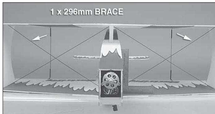
❑ 2. Install the 1 x 296mm carbon rods in the wings as shown. Square the fuselage with the wing and glue the wing braces in place.
