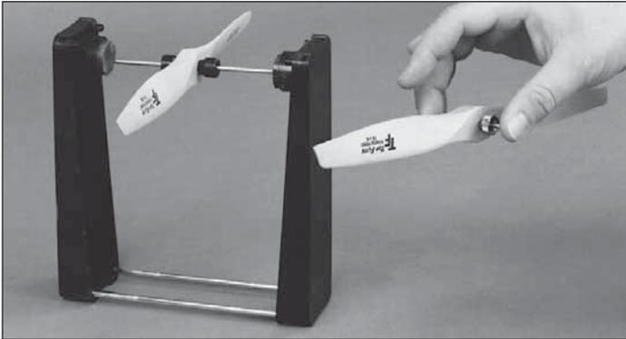
Carefully balance your propeller and spare propellers before you fly. An unbalanced prop can be the single most significant cause of vibration that can damage your model. Not only can screws and bolts loosen, possibly with disastrous effect, but vibration may also damage your radio receiver and battery.
