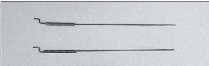
❑ 5. Locate the two 1 x 112mm carbon aileron pushrods, four pieces of heat shrink tubing, and the remaining four Z-bends. Assemble one end of the pushrods as shown.
