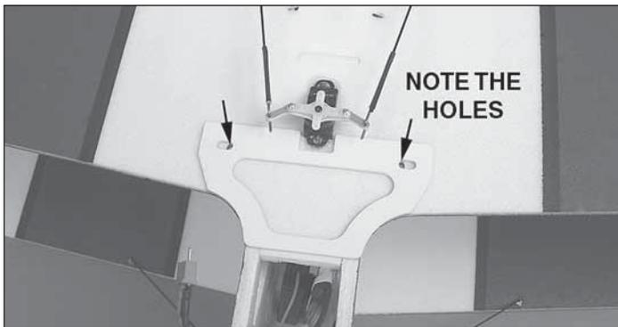
❑ 4. Apply several generous beads of medium or thick foam-safe CA to the back side of the landing gear doubler (the side you just sanded). Center the doubler over the holes in the bottom of the lower wing and glue it in place.
