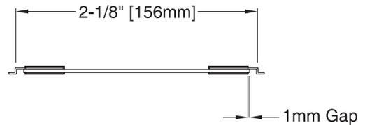
❑ 1. Locate four 1 x 145mm carbon pushrods, eight 1 x 30mm Z-bends, and eight 25mm pieces of heat shrink tubing. Assemble four **aileron link rods** as shown in the sketch above so that they measure 2-1/8" [156mm] from Z-bend center to Z-bend center. See the **Expert Tip** below on how to assemble pushrods.
