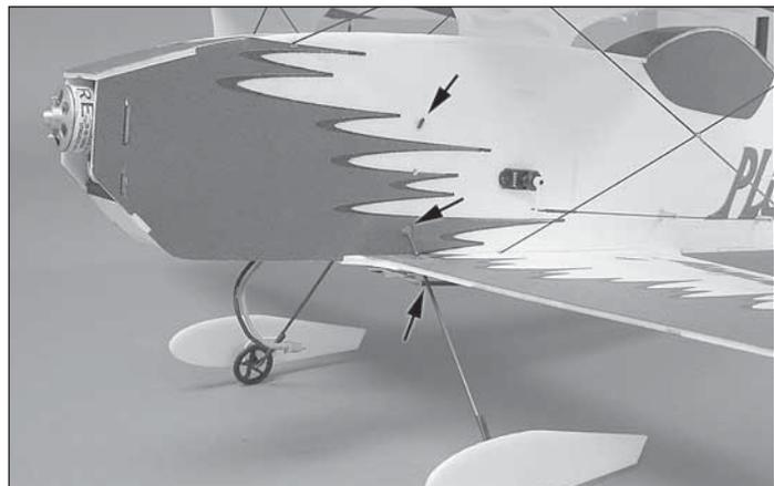
❑ 7. Slide each landing gear leg through the holes provided in the wing. They will go through the wing holes first, then the fuselage side, and then cross over to the opposite fuselage side. Rotate the landing gear rod until the wheels point straight ahead. Glue the landing gear in place.
