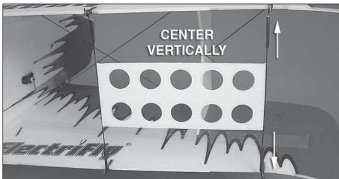
❑ 10. Speed brakes have been provided for you if you fly indoors. These are optional and should not be installed until the model has been test-flown and properly trimmed out. Install them between the aileron link rods so that they are centered vertically. Use thick foam-safe CA or tape to attach these to the link rods. These should only be used indoors and will help keep speed constant during up and downline maneuvers.
