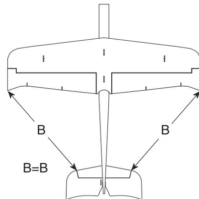
❑ 2. Align the stab vertically and horizontally as shown in the sketches above. If the stab doesn't sit parallel with the plane
