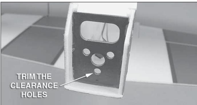
❑ 2. Test fit your motor by holding it in place up against the firewall. Make sure that the Y-mount screws fit inside of the clearance holes in the firewall. If it is necessary, carefully enlarge the holes using a Dremel® tool or a sharp hobby knife.
