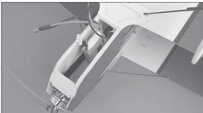
❑ 1. Place the battery pack in the plane. **Do not** connect the battery to the ESC.
