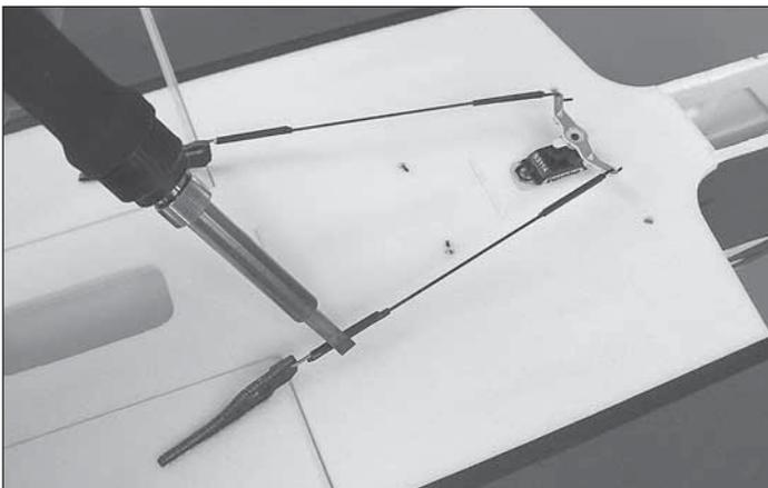
❑ 7. Fit the pushrods to the servo arm. Fit the remaining Z-bends to the aileron control horns and slide a piece of heat shrink tubing onto the carbon rods. Shrink the tubing with a hot soldering iron, making sure that your ailerons stay centered in the process.
