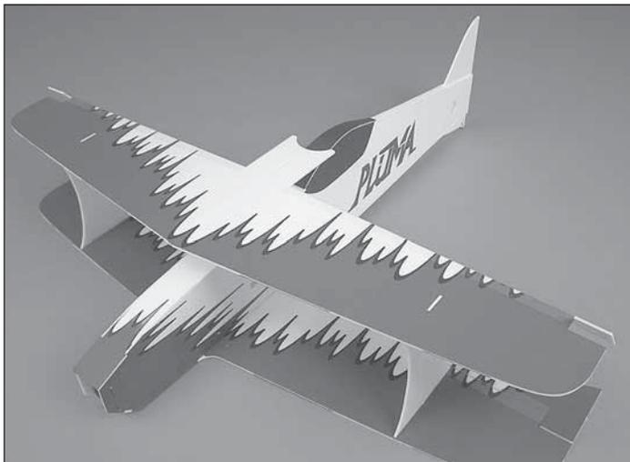
❑ 3. Apply thin foam-safe CA to the tabs on the interplane struts and the center cabane strut. Install the top wing.
