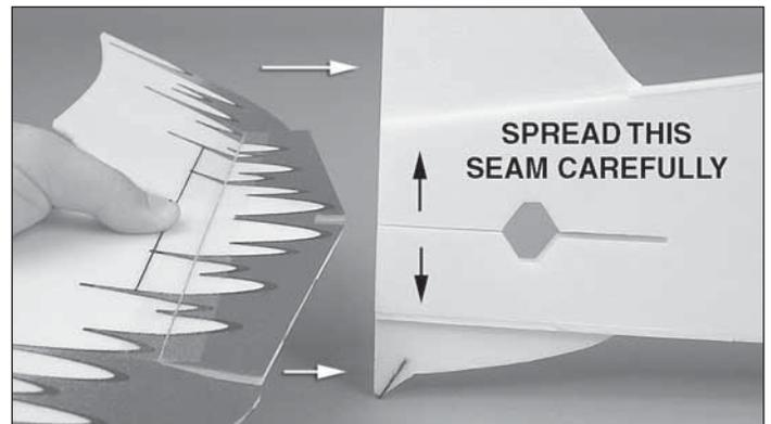
❑ 1. Test fit the horizontal stab to the fuselage, installing it from the rear. You'll need to spread the fuselage seam apart a bit to get the stab in, so use care.
