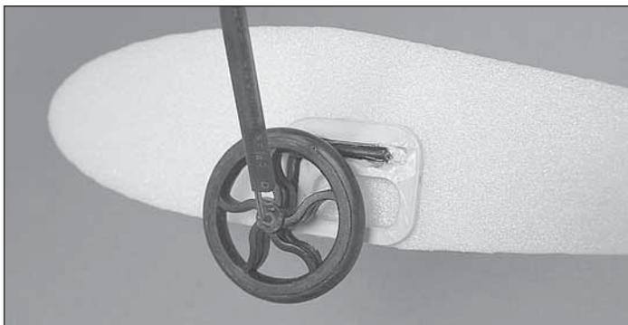
❑ 6. Use medium or thick foam-safe CA to attach the wheel pants to the landing gear legs.
