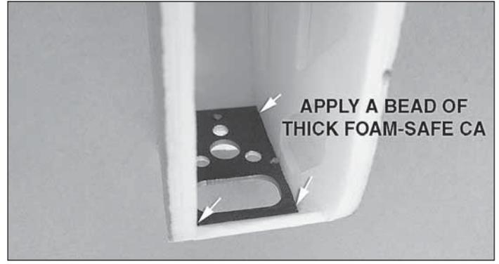
❑ 3. If you are installing the more powerful RimFire motor, apply a bead of thick foam-safe CA to the fuselage-to-firewall joint.
