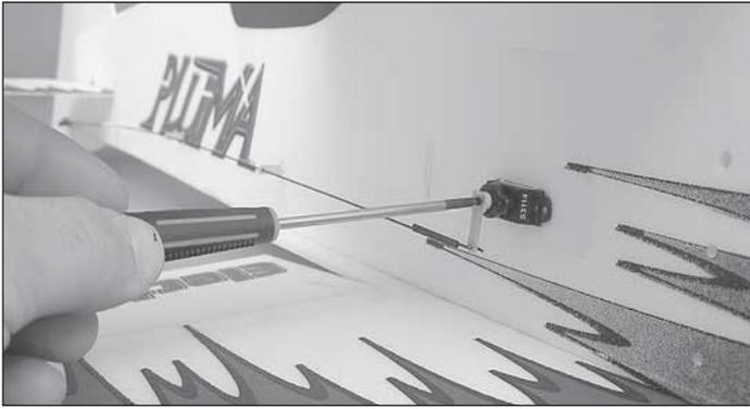
❑ 7. Install the servo arm screws.
