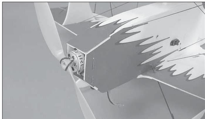
❑ 8. Mount the recommended propeller using a prop saver O-ring. Please see the ***“Motor, Propeller, Battery, & ESC Recommendations”*** section on page 3 of this manual to match the correct prop to your motor.
