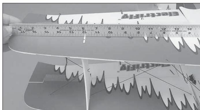
❑ 3. Locate the four 1 x 135mm outer wing braces. Two will be used for the left wing and two for the right wing. With the braces fitted and the lower wing still flat on the table, hold a straightedged ruler against the top wing. Align the wings and glue the braces in place.
