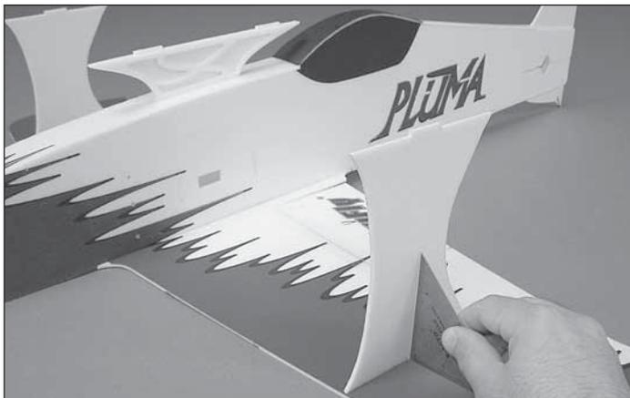
❑ 2. Glue the interplane struts to the bottom wings using thin foam-safe CA. Use a 90° builder's square or the template provided in the back of this manual to properly align the interplane struts vertically. **Note:** The front edge of the interplane struts has less curvature than the aft edge.
