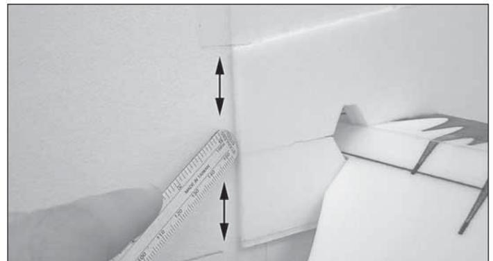
3. Apply the 70mm piece to the center section of the rudder, making sure that you press the tape tightly into the crease. A straightedge is helpful here.
