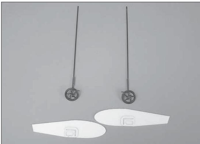
❑ 5. Locate the two pre-assembled landing gear legs and the two foam wheel pants. You should have a right and a left side of each of these.
