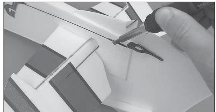
4. Fit the servo arm onto the rudder servo and extend the pushrod all the way back to the rudder control horn. Fit a Z-bend to the rudder control horn. Attach the Z-bend to the rudder pushrod using a 25mm piece of heat shrink tubing. Shrink the tubing with a hot soldering iron. **Note: DO NOT attempt to use a torch, cigarette lighter or heat gun near the foam!** It is nearly impossible to use these without melting the foam.
