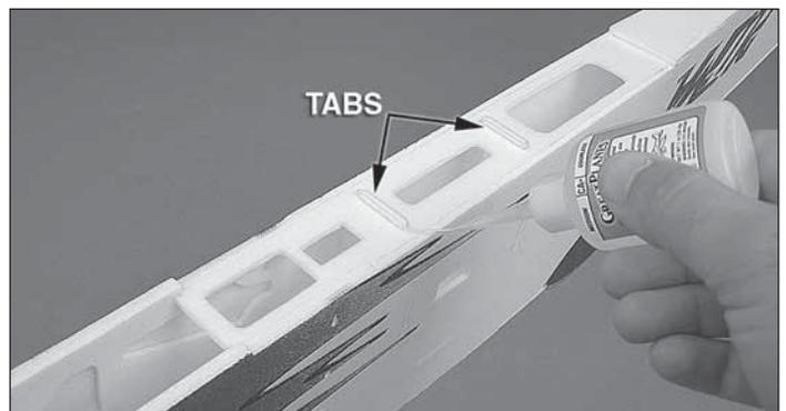
1. Glue the bottom wing to the bottom of the fuselage. Apply a bead of medium or thick foam-safe CA to the wing saddle and the two fuselage former tabs and mount the wing. **Note:** The bottom wing can be identified by the servo hole and the protruding LE stop.
