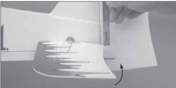
Use a ruler or the templates provided in the back of this manual to accurately measure and set the control throw of each control surface as indicated in the chart that follows. If your radio does not have dual rates, we recommend setting the throws at the **low rate** setting. **Note:** The throws are measured at the **widest part** (inboard or lowest part) of the elevators, ailerons, and rudder.
