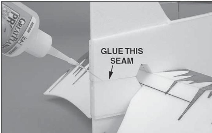
4. Make sure that the upper and lower fuselage is aligned. Apply a few drops of foam-safe CA to the aft fuselage seam and glue the seam together.
