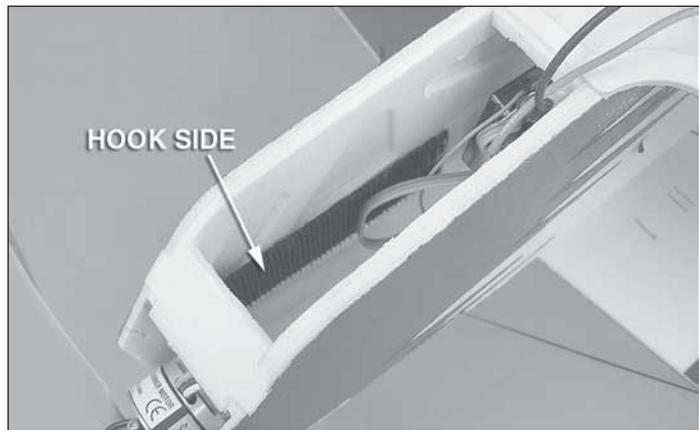
❑ 9. With the hook and loop material that you have left over, separate the hook side from the loop side and stick the hook side (bristly side) inside the fuselage. Apply the remaining loop material to your battery packs.
