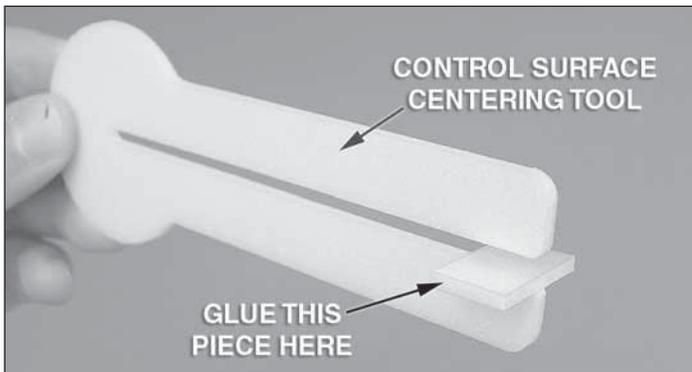
❑ 3. Locate the foam parts shown above and build two control surface alignment tools. **Note:** Setting the rectangular pad at 90 degrees is not critical.
