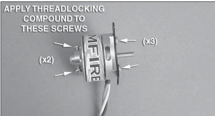
❑ 1. Remove the three screws holding the Y-mount to the back of the motor and the two screws for the prop saver. Apply threadlocking compound to the screw threads and reinstall the screws.
