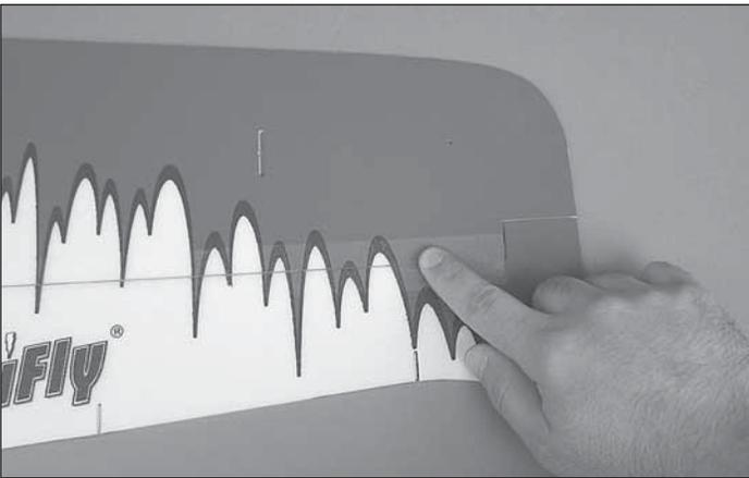
1. Lay the wing panels and horizontal tail on a flat work surface. Gently run your finger over the taped hinges to form a secure bond between the tape and the foam.
