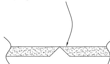
2. Position the rudder so that the LE of the rudder gently touches the vertical fin and that the top of the rudder is even with the top of the fin. Remove the backing paper and apply the 100mm strip of tape to the top of the rudder on the **right side**. Apply the 20mm piece to the bottom of the rudder. **Note:** Pushing the rudder too hard against the fin can fold the beveled edge over and cause limited rudder throw.
