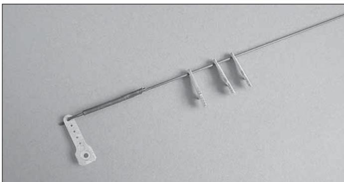
2. Remove the servo arm that you temporarily fitted to your rudder servo. Use a #57 [1mm] drill bit to enlarge the outermost servo arm hole. Fit the rudder pushrod to the outermost hole. **Note:** If you don't have a #57 drill bit, carefully use your hobby knife to enlarge the hole.
