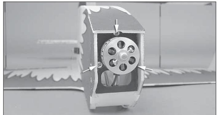
❑ 4. Install the motor using three 2.5 x 8mm self-tapping screws. Remove the screws and the motor and harden the screw holes with one drop of thin regular CA. Be careful not to drip any regular CA onto the foam.
