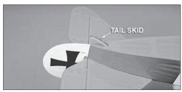
☐ 11. Test fit the tail skid at the rear of the fuse. When satisfied with the fit, attach the tail skid to the bottom of the fuse using medium CA.
