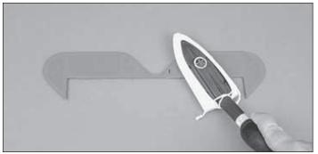
□ 2. Carefully separate the ailerons from the wing, the rudder from the fin and the elevator from the stabilizer (stab). If necessary, use a covering iron set on medium/high to carefully tighten the covering. Lay the control surface on a flat surface and apply pressure over sheeted areas to thoroughly bond the covering to the wood. Hint: Poke three or four pin holes in the covering over the open structure in the tail surfaces. This will allow the hot air to escape while tightening the covering.
