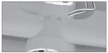
☐ 3. Locate the ABS wing fairing. Trim the front and back as needed for a good fit. Use medium CA to secure it in place as shown.
