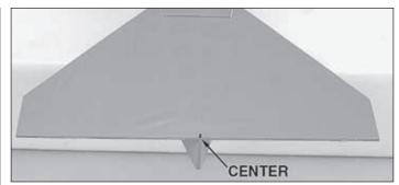
2. Mark the center of the TE of the stab. Place the stab onto the stab saddle.
