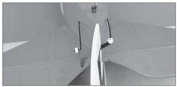
□ 3. Insert the 90° bends of the 460mm [18"] pushrods into the outer hole of the control horns and secure them with the plastic retainers as shown. Place a drop of CA on the outer surface of the plastic retainers.
