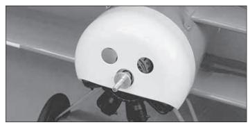
☐ 2. Slide the prop shaft and collet onto the motor shaft. The collet has a tapered hole through it.
