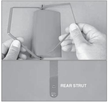
☐ 1. Carefully thread the axle through the sub-wing and attach the rear landing gear strut followed by the front landing gear strut as shown. The rear strut is identified by a second hole near the axle hole.
