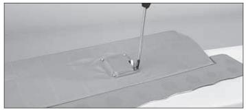
☐ 10. Secure each aileron servo hatch to the wing with four 2mm x 6mm [5/64" x 15/64"] self-tapping washer head screws.
