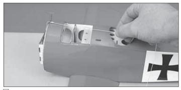
☐ 3. Stick a T-pin into the center of the top of the firewall. Tie a small loop in one end of a 900mm [35"] piece of non-elastic string such as K&S #801 Kevlar thread. Slip the loop in the string over the T-pin.
