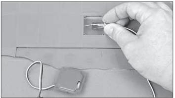
☐ 6. Inside the aileron servo bays of the top wing, there is a string that runs from one bay to the other. Plug the left aileron servo into a 610mm [24"] Y-harness and tie the string around the right aileron servo plug. Be sure to secure the left aileron servo connection with heat-shrink tubing.
