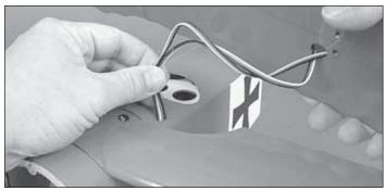
☐ 14. Run the Y-harness receiver plug from the top wing through the slot on the top of the fuse and plug it into the appropriate receiver channel. Re-install the bottom wing.
