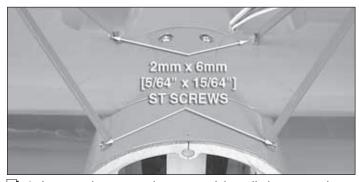
☐ 4. Locate the two cabanes and install them as shown using four 2mm x 6mm [5/64" x 15/64"] self-tapping screws as shown. Remove the screws and apply a couple of drops of thin CA into each hole to harden the threads. Re-install the cabanes.
