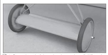
☐ 4. On each end of the axle, place a 3mm [1/8"] washer and 3mm [1/8"] nut with threadlocker, followed by another 3mm [1/8"] washer and the wheel. Secure the wheel in place with a 3mm [1/8"] washer and 3mm [1/8"] nut. Apply a drop of threadlocker to the nut.
