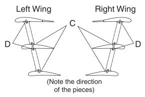
☐ 6. Study the above drawing carefully. It shows the direction and placement of the remaining 8 strut mounts and the four struts. Be sure to insert and remove a 2mm x 6mm [5/64" x 15/64"] self-tapping screw through each one and apply thin CA into each hole to harden the threads.
