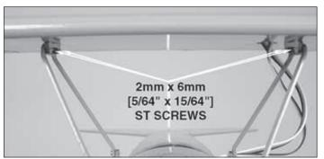
☐ 5. Put the top wing in place atop the cabanes and secure it with four 2mm x 6mm [5/64" x 15/64"] self-tapping screws. Remove the screws and apply a couple of drops of thin CA into each hole to harden the threads. Re-install the top wing.
