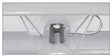
☐ 1. Remove a 13mm x 13mm [1/2" x 1/2"] square of covering from the top of the fuse in front of the cockpit and use CA to attach the machine gun mount. Glue the machine guns in place as shown.
