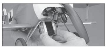
☐ 1. Cut a 20mm [3/4"] long piece of hook and loop material (not included). Glue the rough piece (hook side) to the battery tray. Glue the 20mm [3/4"] soft piece (loop side) to the back of the battery pack. Insert the battery into the battery compartment and secure it in place by joining the hook and loop material.
