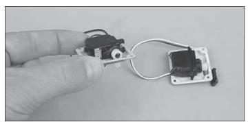
□ 5. Clean the cases of both aileron servos with denatured alcohol. Use CA to glue the aileron servos on the bottom of the aileron servo hatches so that the servo arm is centered in the opening. Cut off all of the unused servo arms as you did in Step 1. If you prefer, wrap electrical tape or heat-shrink tubing around the servos before gluing them to the servo hatch. This will allow the servos to be removed easily.
