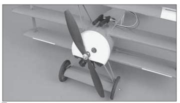
☐ 3. Install a 10" x 4.5" propeller. Install the prop washer and prop nut and tighten the nut securely.
