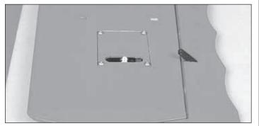
☐ 11. Test fit the control horns into the small rectangular holes along the LE of the bottom of each aileron as shown. When satisfied with their fit, CA them in place as shown.
