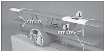
☐ 7. Use 2mm x 6mm [5/64" x 15/64"] self-tapping screws to secure the struts as shown.
