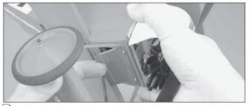
2. Put the battery cover in place. Note that the lip slides into the fuse and the aft end is held on with two magnets.
