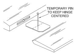
☐ 1. Test fit the right aileron to the top wing with three 5mm x 10mm [13/64" x 3/8"] hinges. If the hinges don't stay centered, stick a pin through the middle of the hinges to hold them in position while fitting the aileron to the wing.
