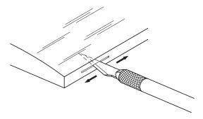
☐ 3. Check the pre-cut hinge slots of all control surfaces using a hobby knife with a #11 blade. This will help when installing the hinges.
