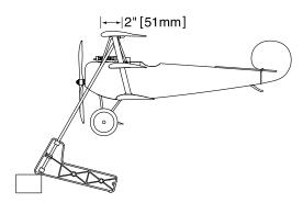
☐ 2. If you are balancing the Fokker DR-1 EP ARF on the Great Planes CG Machine, you will find that the angle of the supports does not allow you to rest the plane forward enough to reach the balance point. To remedy this, simply place the front of the CG Machine on a raised surface (approx. 2" [51mm]). This will allow the plane to be placed further forward on the balancer.
