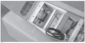
□ 5. Cut another 20mm [3/4"] long piece of hook and loop material (not included) and glue the 20mm [3/4"] soft piece (loop side) to the back of the receiver. Glue the rough piece (hook side) to the top of the inside of the fuse on the ledge by the cockpit opening. Insert the receiver and secure it in place by joining the hook and loop material.
