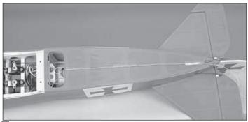
☐ 13. Make a small hole in the bottom sheeting. Route the antenna out of the hole and tape it to the bottom of the fuse with clear tape.
