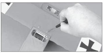
☐ 2. Test fit the bottom wing to the fuse and secure it with two 3mm x 24mm [1/8" x 15/16"] machine screws and 3mm [1/8"] washers. The flat side of the wing is the bottom.
