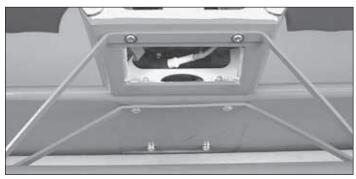
☐ 3. Attach the landing gear to the bottom of the fuse with four 2mm x 7mm [5/64" x 9/32"] self-tapping washer head screws. Remove the screws and harden the holes with thin CA. Then, reinstall the screws.
