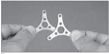
☐ 1. Use epoxy to join the two piece motor mount. Make sure all openings align.
