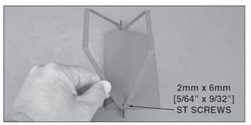
☐ 2. Secure the sub-wing to the landing gear with two 2mm x 6mm [5/64" x 15/64"] self-tapping screws as shown. Remove the screws and harden the holes with thin CA. Then, reinstall the screws.
