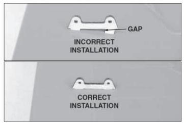
☐ 2. Grab the two strut mounts that you marked "A" and insert them into the pockets on the top wing as shown. They are designed to fit only one way. If you observe a large gap between the wing and strut mount, remove it and try it the other way. **DO NOT** glue them into place at this time.
