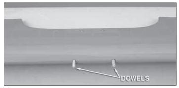
☐ 1. Locate the two remaining 3mm x 24mm [1/8" x 15/16"] dowel rods and insert them into the middle wing as shown, so that only about 9mm [11/32"] sticks out. Secure them with medium CA.
