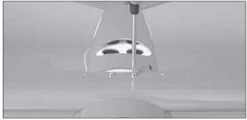
☐ 2. Place the middle wing on the wing saddle as shown and secure it with two 3mm x 24mm [1/8" x 15/16"] machine screws and 3mm [1/8"] washers. The flat side of the wing is the bottom.
