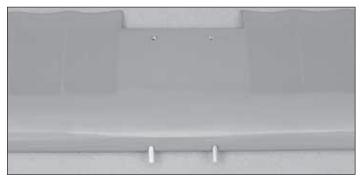
☐ 1. Locate two of the 3mm x 24mm [1/8" x 15/16"] dowel rods and insert them into the bottom wing as shown, so that only about 9mm [11/32"] sticks out. Secure them with medium CA.
