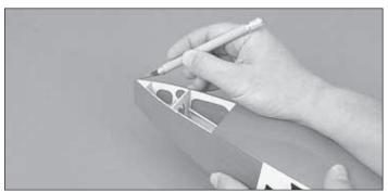
☐ 1. Using a sharp hobby knife, remove the covering from the stab cut-out at the aft end of the fuse.
