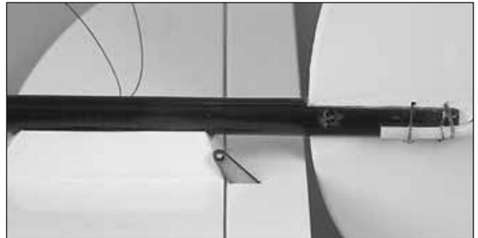
2. Slide the single sided plywood control horn into the elevator and glue with thin CA.
