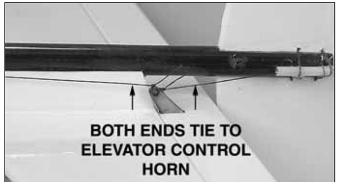
10. Tie the cut ends of the string to the elevator control horn. The strings need to have some tension on them and the elevator needs to be aligned with the stab. After you have confirmed that the elevator is straight and moves full throw of the servo secure the knots with a drop of thin CA.
