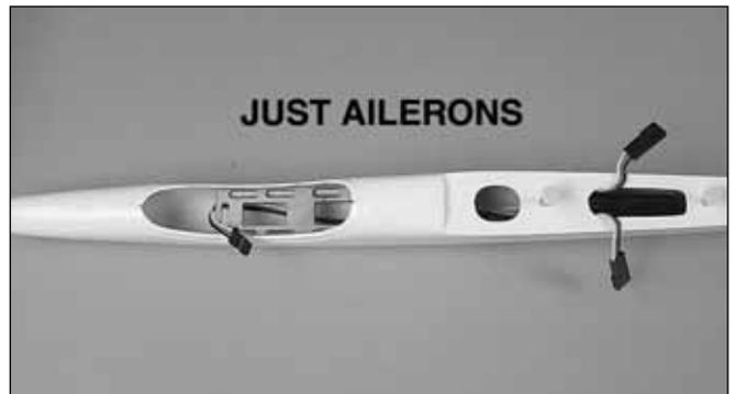
3. Install the aileron extensions under the servo tray.
