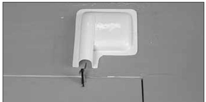
8. Trim the plastic aileron servo cover and place over the servo. Check that the cover does not interfere with the movement of the servo. Tape the cover to the wing.
