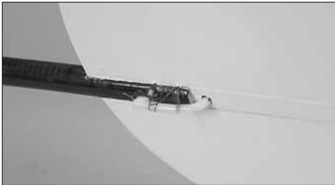
8. Pull the remaining string through the rear hole and loop it around the fuse and elevator turnaround as many times as possible. Pull the string tight and secure it with thin CA.
