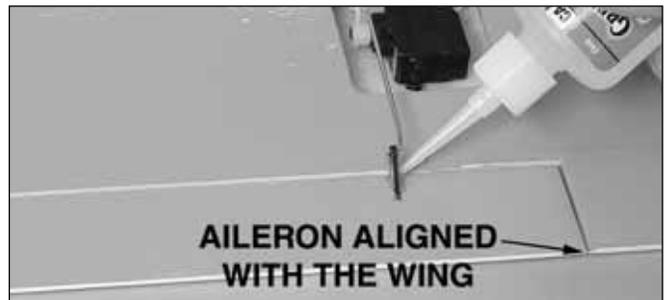
7. Cut the covering from the control horn slot on the bottom of the aileron. Fit the plywood control horn to the pushrod. Fit the control horn in the slot. Make sure that the arm is centered with the radio on and the trim centered. Align the aileron TE and wing TE, then glue the control horn to the aileron with thin CA.
