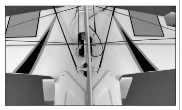
□ 21. Insert the z-bend of both **aileron pushrods** in the anti-differential arm.
