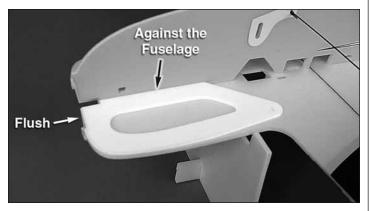
□ 23. Turn the plane upside down and glue the two **horizontal fuselage doublers** to the front of the fuselage. Make sure they are flush with the front of the fuselage and against the vertical fuselage.
