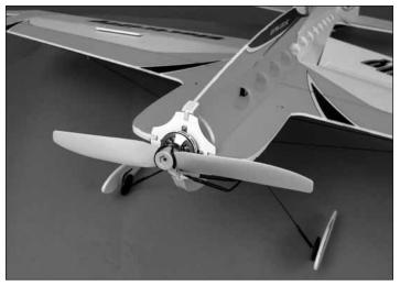
□ 7. Install the propeller on the motor following the motor instructions. **Hint:** The rubber o-ring can be difficult to stretch over the screw, then the propeller and over the other screw. A small jewelers phillips head screwdriver can be used to pry the rubber o-ring over the screws and propeller. Be careful not to allow the screwdriver to slip and damage the windings inside the motor.
