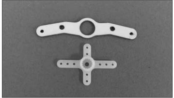
□ 17. Locate the **anti-differential arm**. Place the antidifferential arm on the underside of the servo arm. If you are using Futaba servo arms, the holes in the servo arm and the holes in the anti-differential arm will align. If you are using another brand of servo arm, you will need to use a #60 [1mm] drill bit to drill a pilot hole through the servo arm that will align the servo arm with the anti-differential arm.
