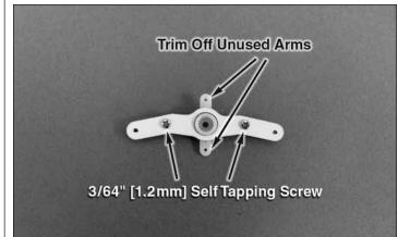
□ 18. Attach the anti-differential arm to the servo arm using two 3/64" [1.2mm] self tapping screws.
