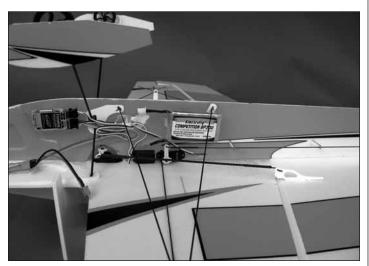
□ 4. Apply the remaining hook and loop material to the side of the fuselage at the approximate location for the motor battery. Attach an opposite piece of hook and loop material to the battery. Trial fit the motor battery to the side of the fuselage and recheck the CG.
