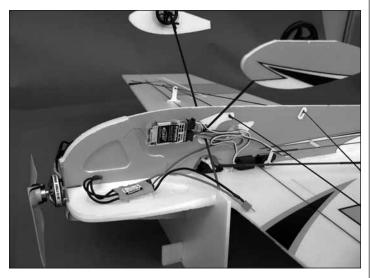
□ 6. Position the receiver on the side of the fuselage, under the wing as far forward as possible. Make sure that the servo wires do not interfere with the pushrods. Apply a piece of hook material on the side of the fuselage, at the receiver location. Attach the receiver to the fuselage. To prevent the wires from interfering with the pushrods, use a small piece of tape to attach them to the fuselage.
