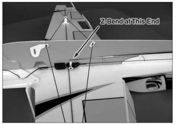
□ 10. Insert the **rudder pushrod**, from the front, through the five pushrod guides. The z-bend should be next to the rudder servo arm.
