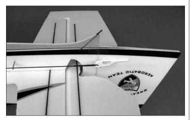
□ 12. Slide the **black heat shrink tubing** over the aft end of the rudder pushrod. Insert the **z-bend wire** into the hole in the **rudder control horn** from the bottom. Slide the other end of the z-bend wire into the heat shrink and install the rudder control horn in the rudder. **Note:** The rudder hinge tape may be covering the front of the rudder control horn slot. Use a sharp hobby knife to trim the tape from the slot.
