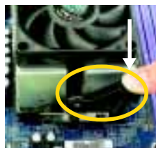
Figure 5&6. Alignment of Heatsink Assembly with Standoffs
