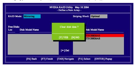
Press **Y** if you want to wipe out all the data from the RAID array, otherwise press **N**. You must choose **Yes** if the drives were previously used as RAID drives. The **Array List** window appears, where you can review the RAID arrays that you have set up.
