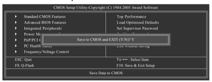
Type "Y" will quit the Setup Utility and save the user setup value to RTC CMOS.
