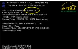
Press Del to enter BIOS menu after system reboots and "Load BIOS Fail-Safe Defaults". See how to Load BIOS Fail-Safe Defaults, please kindly refer to Step 6 to 7 in Part One.
