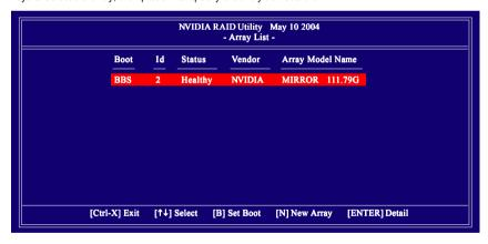
Press Enter to view and verify details. The Array Detail screen appears.
