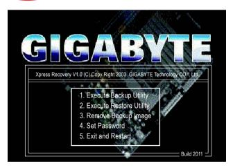
2. Press F9 during powering on the computer. (Text Mode)
