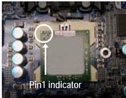
3. Locate Pin 1 in the socket and look for a (golden) cut edge on the CPU upper corner. Then insert the CPU into the socket.
