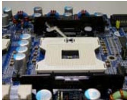
1. Angling the rod to 65-degree maybe feel a kind of tight , and then continue pull the rod to 90-degree when a noise "cough" made.
