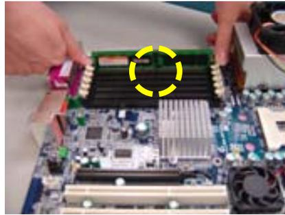
2. Insert the DIMM memory module vertically into the DIMM slot. Then push it down. Please note that DIMM must be populated in order starting at the nearest slot from the ATX power.
