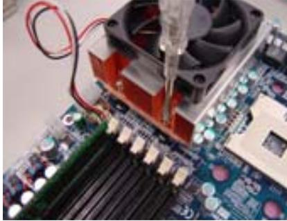
3. Fasten the heatsink supporting-base onto the CPU socket on the mainboard.
