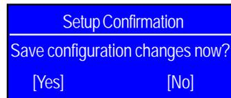
Press [Yes] to save setup data to CMOS.
