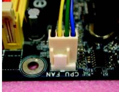
4. Make sure the CPU fan is plugged to the CPU fan connector, than install complete.
