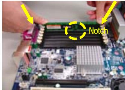
3. Close the plastic clip at both edges of the DIMM slots to lock the DIMM module. Reverse the installation steps when you wish to remove the DIMM module.
