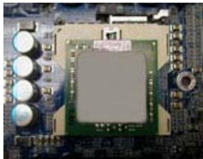
4. Press down the CPU socket lever and finish CPU installation.
