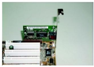
Figure A: Standard CNR Card
