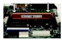
Insert the RIMM module into the slot.
