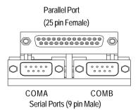
➤ This connector supports 2 standard COM ports and 1 Parallel port. Device like printer can be connected to Parallel port; mouse and modem etc can be connected to Serial ports.
