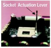
1. Pull up the CPU socket level and up to 90-degree angle.
