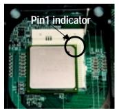
Locate Pin 1 in the socket and look for a (golden) cut edge on the CPU upper corner. Then insert the CPU into the socket.
