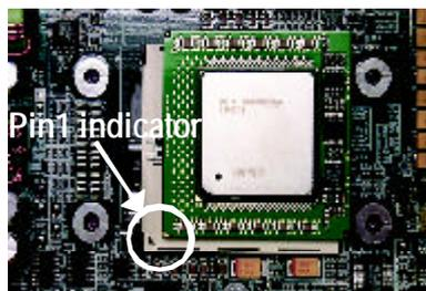
2. Locate Pin 1 in the socket and look for a (golden) cut edge on the CPU upper corner. Then insert the CPU into the socket.
