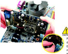
Please carefully pull out the small whitedrawable bar at the end of the PCI Express x 16 slot when you try to install/Uninstall the VGA card. Please align the VGA card to the onboard PCI Express x 16 slot and press firmly down on the slot .Make sure your VGA card is locked by the small white-drawable bar.
