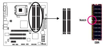
1. The DIMM slot has a notch, so the DIMM memory module can only fit in one direction.
