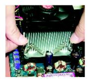
Hook one end of the cooler bracket to the CPU socket first.
