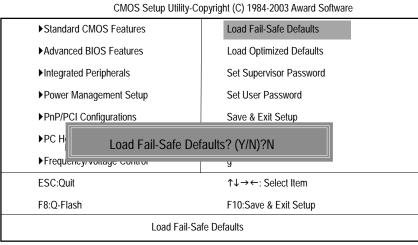
Figure 9: Load Fail-Safe Defaults
