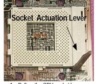
1. Pull up the CPU socket lever and up to 90-degree angle.
