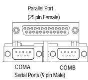
This connector supports 2 standard COM ports and 1 Parallel port. Device like printer can be connected to Parallel port; mouse and modem etc can be connected to Serial ports.
