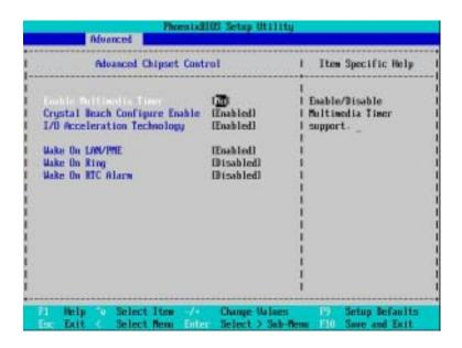
Figure 2-4: Advanced Chipset Control
