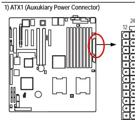
AC power cord should only be connected to your power supply unit after ATX power cable and other related devices are firmly connected to the mainboard.
