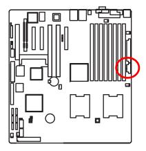
➤This connector (ATX +12V) is used only for CPU Core Voltage.
