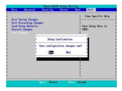
Press [Yes] to save setup daya to CMOS.
