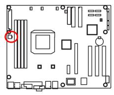
➤This connector (ATX +12V) is used only for CPU1 Core Voltage.
