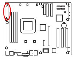
AC power cord should only be connected to your power supply unit after ATX power cable and other related devices are firmly connected to the mainboard.
