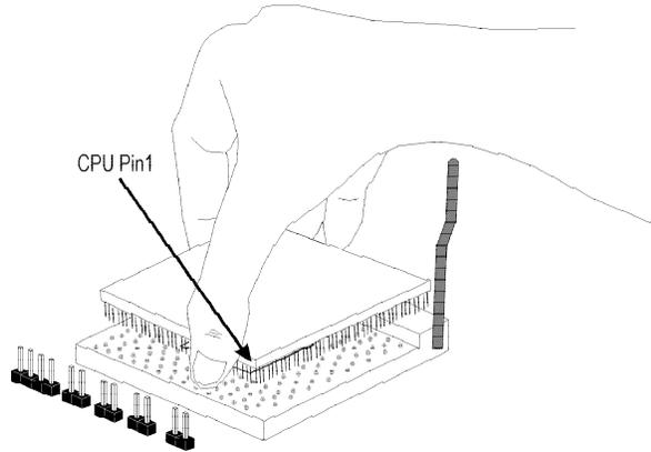
**Positioning the CPU Above the ZIF Socket**
