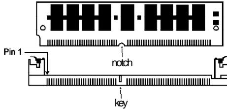
1. Position the SIMM above the socket with the “notch” in the module aligned with the “key” on the socket.
