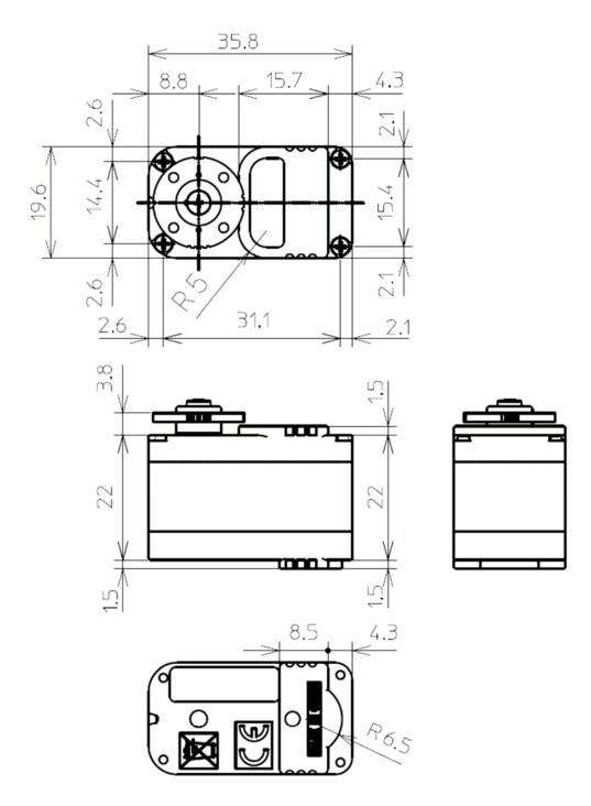
Figure 0-1 Dimensions with using Joint-Ball
