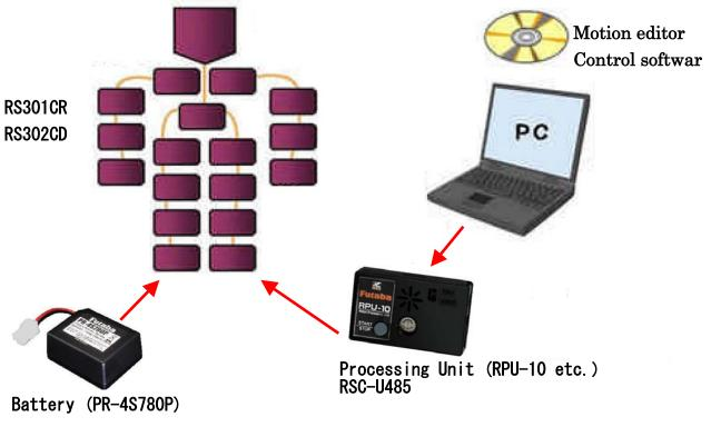
Fig. 3.1 Robotic system configuration
