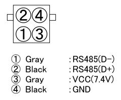
Fig. 3.2 Pin assignment
