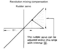
When this compensation is suitably applied, the high speed linearity in the air is improved and power loss is minimized.
