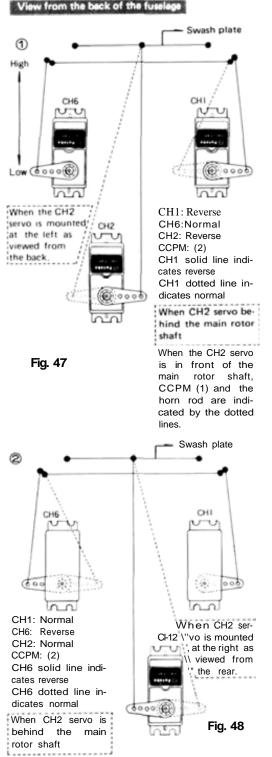
When the CH2 servo is in front of the main rotor shaft, CCPM (1) and the horn rod are indicated by the dotted lines.
