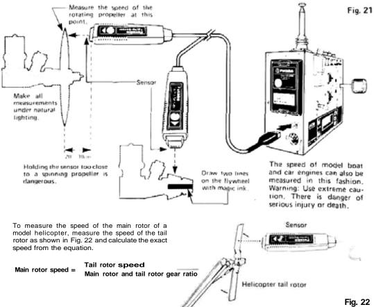
Make all speed measurements outdoors under natural lighting. Accurate speed measurements cannot be made
