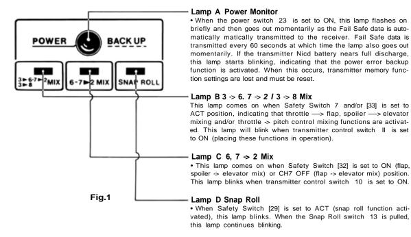
When the power switch 23 is set to ON, lamp (A) will go out momentarily. This indicates automatic data transmission on and is not a failure.
