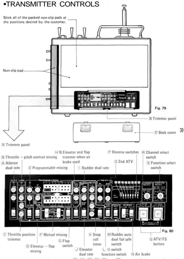
Use the transmitter with fail-safe switches 7, 10, 29, 31, 32, and 33 in the INHIB (function off) position until you become familiar with the set.
