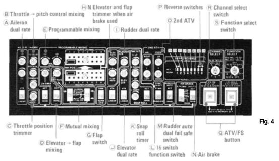
Use the transmitter with fail-safe switches [7], [10], [29], [31], [32], and [33] in the INHIB (function off) position until you become familiar with the set.
