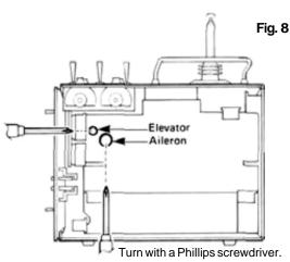
The spring tension can be adjusted as desired by removing the transmitter longer back cover and turning the adjusting screw of each stick. Adjust the spring tension for the best stick feel.
